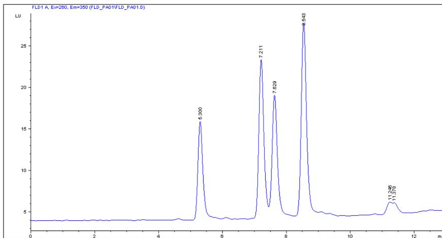
Figure 37 Chromatogram from Emissions Scan
