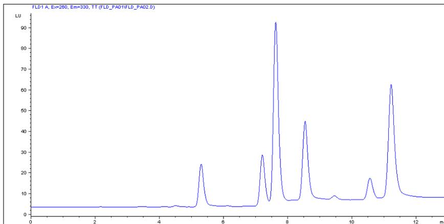
Figure 40 Chromatogram - excitation scan at reference wavelength 260/330 nm
