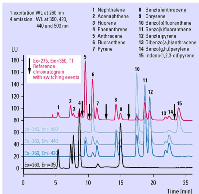
Figure 35 Simultaneous multi wavelength detection for PNA-analysis
