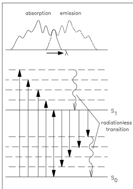
**Figure 3** Relationship of Excitation and Emission Wavelengths
