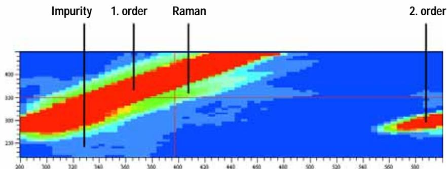
Figure 28 Isofluorescence plot of a mobile phase
