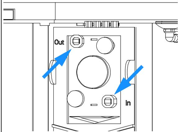
6 Connect the waste tubing to the bottom waste fitting.
