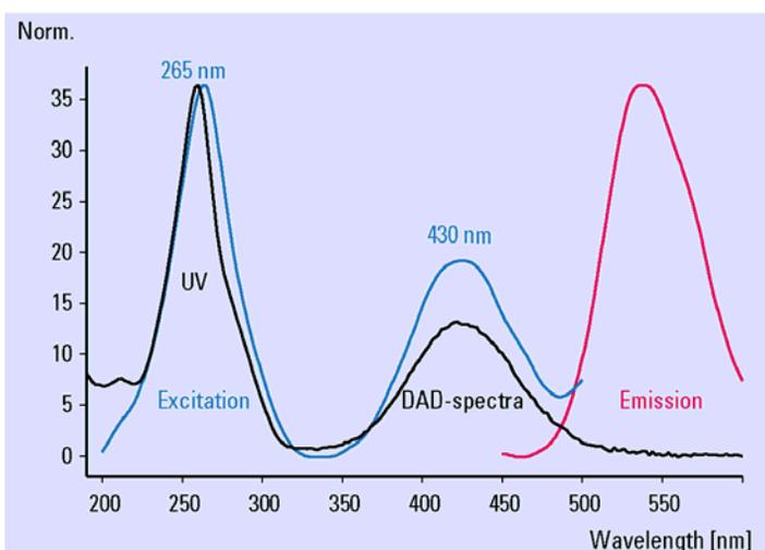
Figure 33 UV-spectrum and fluorescence spectra for 2,3-diaminophenazine (DAP)
