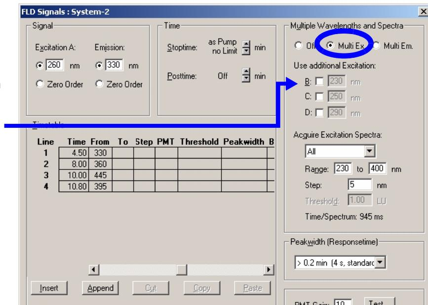
Figure 39 Detector Settings for Excitation Scan
