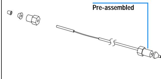
4 Assemble the waste tubing from the accessory kit.
