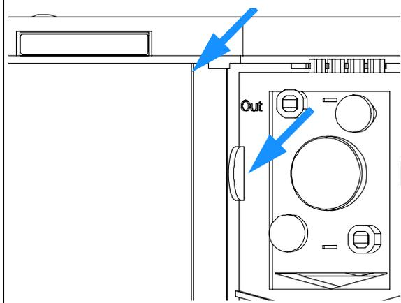
3 Unscrew the thumb screws and pull the flow cell out of the compartment.
