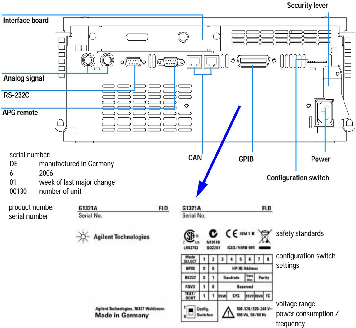
Figure 17 Electrical Connections
