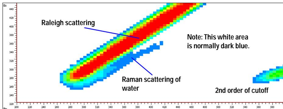
Figure 43 Fluorescence Scan of Water
