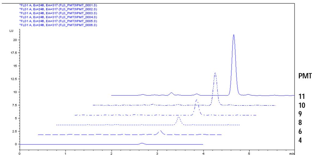
**Figure 45** Finding Best PMTGAIN for Biphenyl
