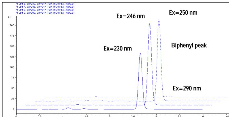
Figure 26 Biphenyl peak with different excitation wavelengths
